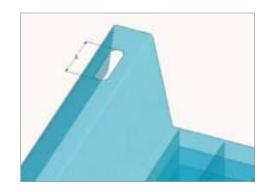
Positioning a **silicone bead**, (preferably special for polycarbonate) on the upper part of the skylight fretwork and on the fretwork of the HI-XT panel and placing the plate between the two HI-XT sandwich panels, which will guarantee leaktightness.
