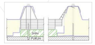
If the HI-XT panel is installed before the skylight leaving a clearance between the HI-XT panels which will be interleaved with the skylight, it is recommended to use a sample of XT LUX to adjust this clearance.
